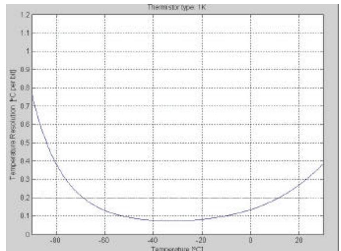
Temperature vs. ADC resolution of  $T_{\text{ambient}}$
