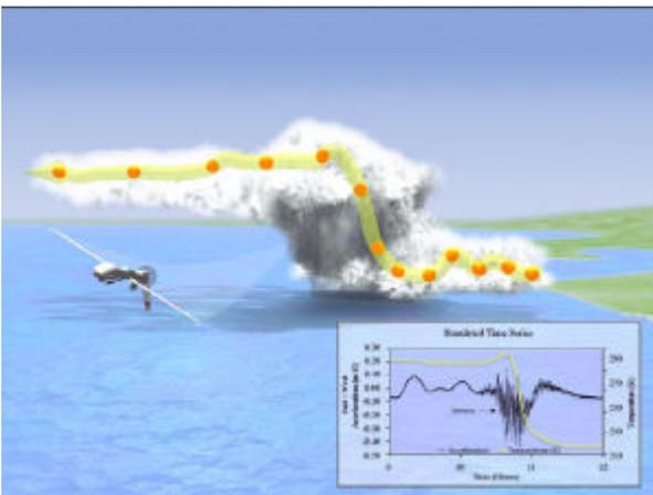
Dropsonde deployment from a UAV
