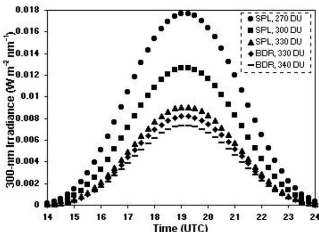
Fig. 6. Model-calculated time series of 300-nm irradiance for 20 June 1999, with variation in ozone column amount at Boulder, Colorado (1.6 km elevation) and at SPL (3.2 km).
