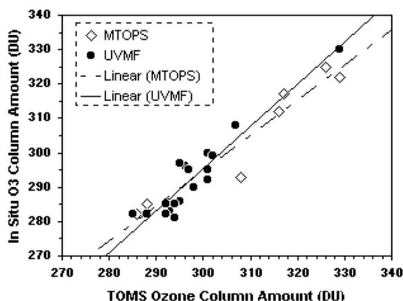
Fig. 4. Intercomparison of ozone column amount obtained from TOMS data with *in situ* retrievals by the UV-MFRSR and the MicroTOPS sunphotometer.
