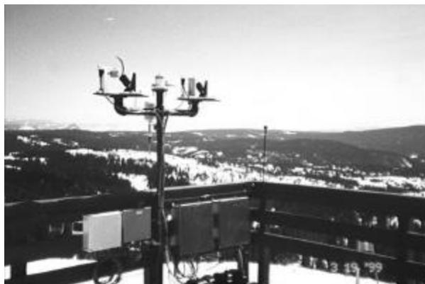
Fig. 2. UV and solar filter radiometer system at Storm Peak Laboratory.
