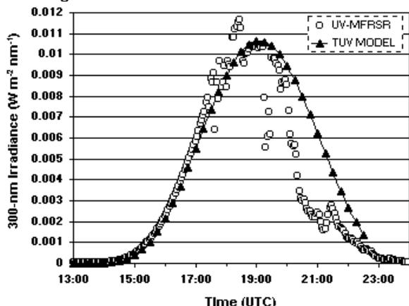
Fig. 8. Comparison of model (TUV) clear-sky and measured (UV-MFRSR) spectral irradiance at 300 nm for 21 April 2000.
