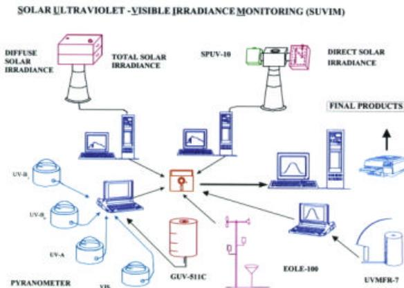
Figure 1. Schematic view of the IASB UV station
