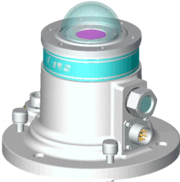
**Solid Model of UV Pyranometer**
