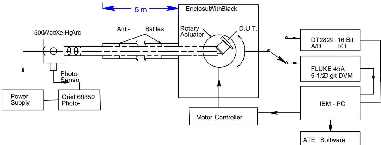
Figure 1. Schematic diagram of the Cosine Response Facility
