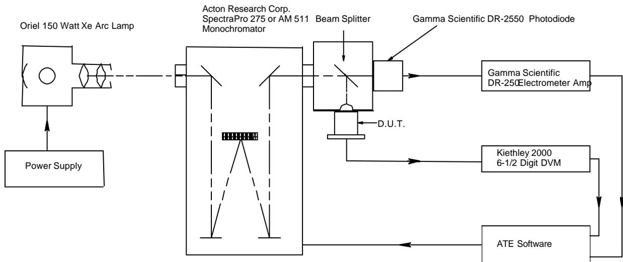
**Figure 2. Schematic diagram of the Spectral Response Facility.**
