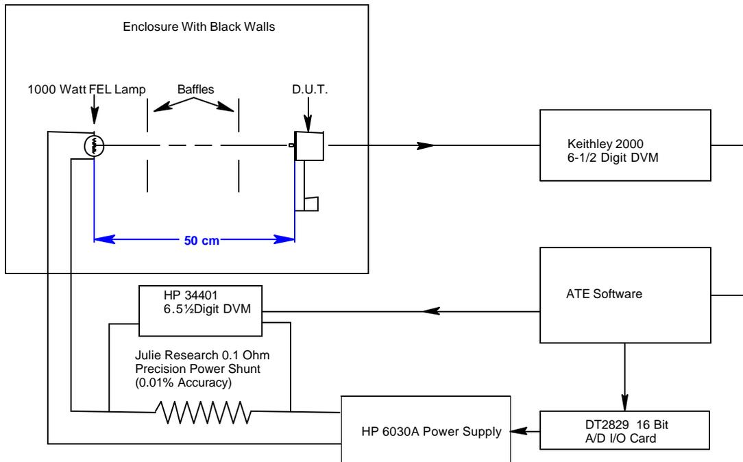
**Figure 3. Schematic diagram of the Absolute Response Facility.**
